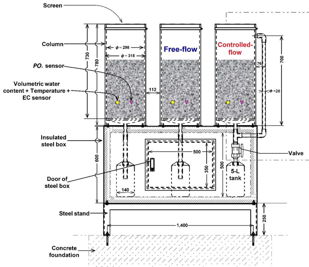
Fig. 1. Schematic diagram of the in situ column experimental setup. Dimensions in this diagram are all in mm.
