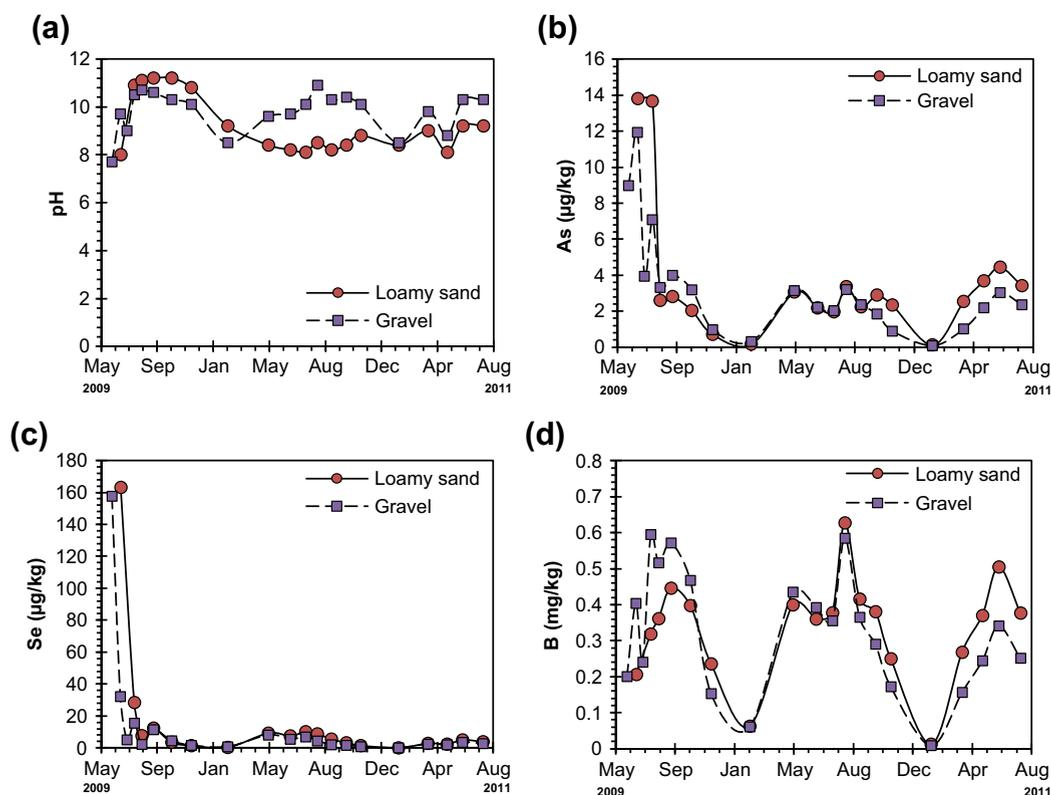
**Fig. 3.** Evolution of effluent pH and the leachabilities of As, Se and B in the columns with loamy sand- and gravel-sized aggregates; (a) effluent pH change with time, (b) change of As leachability with time, (c) change of Se leachability with time, and (d) change of B leachability with time.
