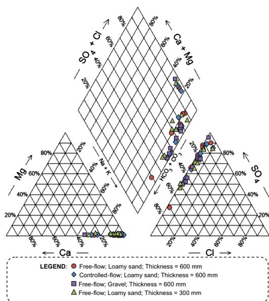
Fig. 5. Piper diagram showing the hydrochemical facies of effluents collected under in situ conditions.
