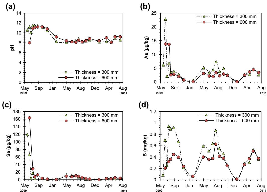
Fig. 4. Evolution of effluent pH and the leachabilities of As, Se and B in the 300 and 600 mm-thick columns; (a) effluent pH change with time, (b) change of As leachability with time, (c) change of Se leachability with time, and (d) change of B leachability with time.
