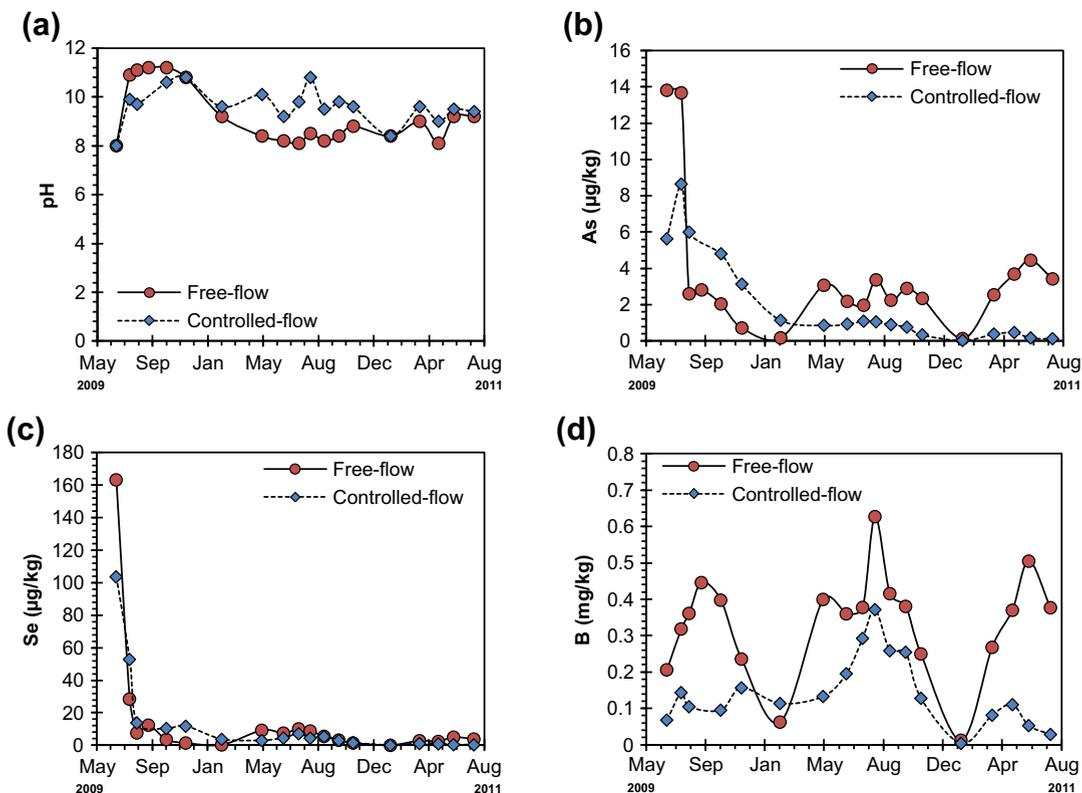
Fig. 2. Evolution of effluent pH and the leachabilities of As, Se and B under free- and controlled-flow conditions; (a) effluent pH change with time, (b) change of As leachability with time, (c) change of Se leachability with time, and (d) change of B leachability with time.
